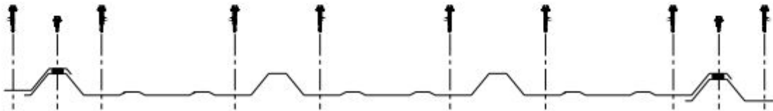
PBR-Panel Fastening Pattern - Ends
