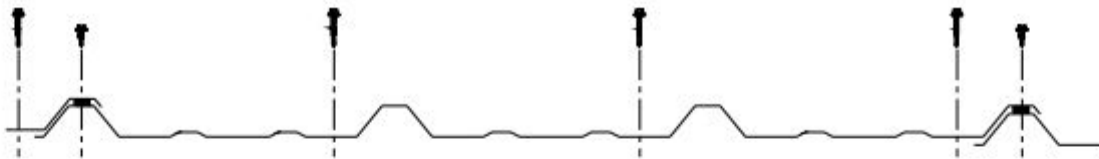
PBR-Panel Fastening Pattern - Interior
